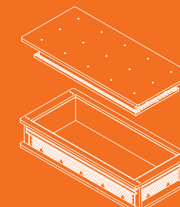
MOLDE GRANDE BIG MOULD 760 x 380 x 190 mm 900 x 380 x 190 mm
